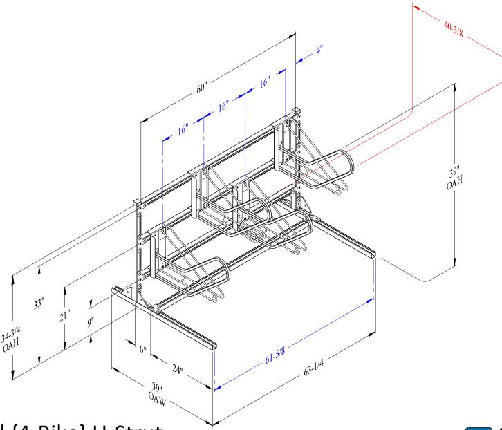
Bike Stall {4-Bike} U-Strut Strut Base {Straight} Assembly {Dim's}
